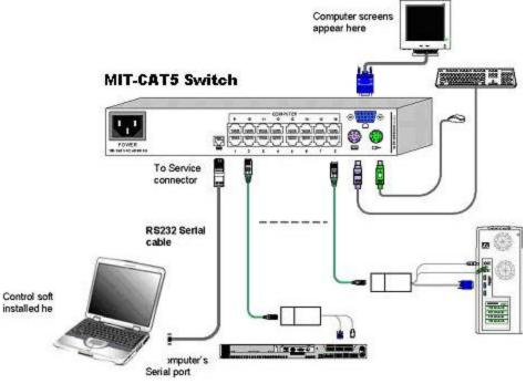
Figure 16 Connecting the RS232 Serial cable
